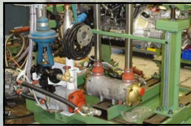
Charge Air and Oil Cooler on an experimental engine test facility.
