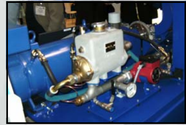
Small Header Tank unit used on fuel testing rig.
