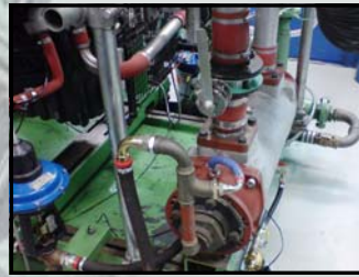
Large Charge Air Cooler assembled on an engine test bed.
