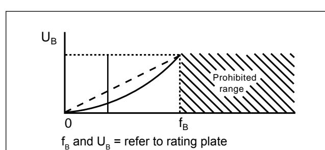
If this is ignored, the motor current will increase disproportionately and the drive motor will fail to achieve its rated speed.
